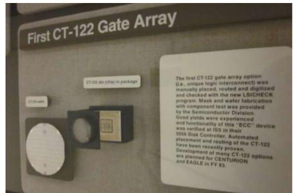
interconnect) was manually placed, routed and digitized and checked with the new LSICHECK program. Mask and wafer fabrication with component test was provided by the Semiconductor Division. Good yields were experienced and functionality of this "ECC" device was verified at ISS in their 5056 Disk Controller. Automated placement and routing of the CT-122 have been recently proven. Developments of many CT-122 options are planned for CENTURION and EAGLE in FY'83.
