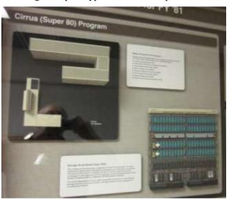
two piece assembly. The basic board section contains common circuitry and 65,536 words of storage. In the expansion to full capacity an outer (blank) portion of the board is replaced with additional 65,536 words of storage. *The board displayed is a test model using DIP connectors*
