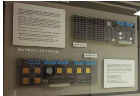
(MSUC) and Interface Controller Chip (ICC) are not part of the Chip-Set. Chip-Set packages included in the IP are: ALU- Arithmetic Logic Unit, AGU- Address Generator Unit, DCD-Decode Control, CIM- Cache Interface Master, EIS- Extended Instruction Set, CIS- Cache Interface Slave(Optional), and M/D- High Speed Multiply /Divide (Optional).
