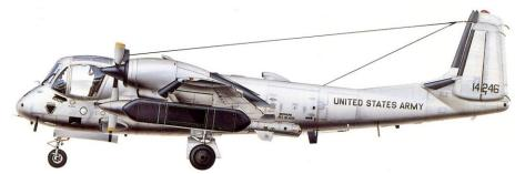
Quicklook II was hosted on the Grumman RV-1D aircraft. This airframe could be repurposed to support different collection platforms. The aircraft had a range of 1,000 miles with two under-wing gas tanks and had a top speed of 330 knots. It could carry a lot of weight and was extremely stable. It was explained to me that what made the RV-1D a great plane for the job is that it was 'slow'; slow makes for a better data collection platform.
