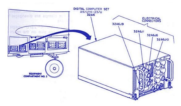
The RV-1D's belly contained two AN/UYK-23 Computers, each AN/UYK-23 having a different mission and designation. The computer designated as the 'CLP' communicated with the Pod. It would tune the frequency of the Pod and then listen for any received signal data from the Pod. The other computer was designated as the 'PCC' and would collect the navigation data from the INS. Data was later extracted from the system and post processed.
