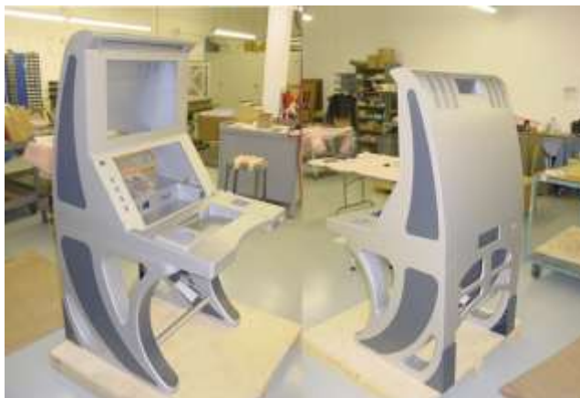
Picture 5. Low-weight two-eye Valiant console designed for P-3C fuselage contour.
