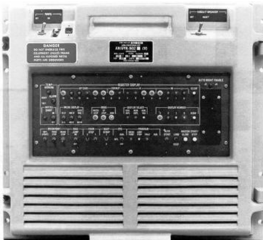
Figure 8. The AN/UYK-502 11 developed in the 70s had typical 16-bit register indicators, whereas the AN/UYK-44 12 in the 80s used a hexadecimal keypad and a small LED screen for internal register readouts, snapshots by Keith Myhre.
