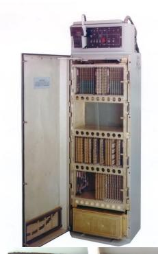
Picture 13B (left) shows the open cabinet with chassis trays and modules. The I/O chassis is on top, the processor chassis is second from the bottom, and the Memory chassis is on the bottom. The last three cards on the right that come out to the edge of the processor tray is the cache memory.
