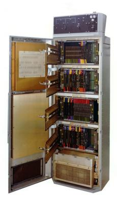
When power was lost the computer would run for 5 minutes and then shut down the logic. The DRAM memory would be held up for an additional 25 minutes.
