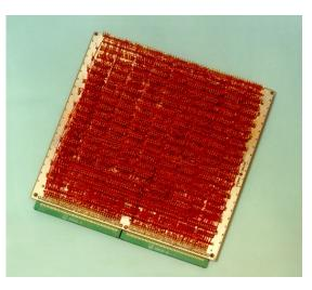
Picture 13I (below) is an I/O adapter module. i.e. Mil-Std-1397 type B. To change I/O interfaces the adapter modules were replaced with the appropriate one. This board also went through the layout process, but was not nearly as successful as the earlier PWB. Note the 30-gauge rework wire running between the chips on the left side.
