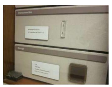
with 9 edge connectors resulted in 16 connections per square inch. The storage was 4,096 bits of core with a cycle time of 2 microseconds and a capacity of 393,210 characters.
