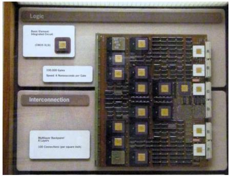
The multilayered back panel had 8 layers and resulted in 100 connections per square inch. The storage uses 256K semiconductor memory devices with a cycle time of 432 nanoseconds and a capacity of 50,331,648 characters.
