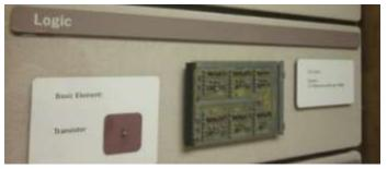
In 1965 the 1108 System had 30,000 gates using transistors. The basic logic element had 50 gates with a speed of 15 nanoseconds per gate.
