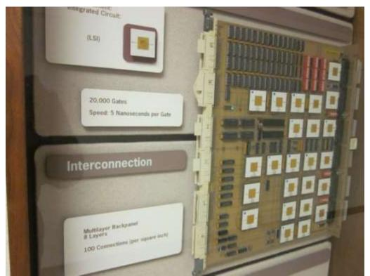
A drawer has 24 LSI and a back panel with 8 layers resulting in 100 connections per square inch. The storage uses 64K semiconductor memory devices with a cycle time of 300 nanoseconds and a capacity of 4,194,304 characters.
