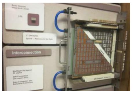
The multilayered back panel has 31 layers with zero insertion force (ZIF) edge and back panel connectors resulting in 200 connections per square inch. The LSI are mounted on both sides of a liquid cold plate.
