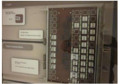
The multilayered back panel has 26 layers and a complete chassis had 28 VLSI and 278 connections per square inch.
