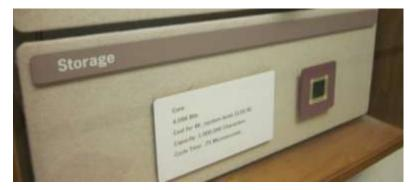
The storage was 4,096 of core with a cycle time of 0.75 microseconds and a capacity of 1,000,000 characters.
