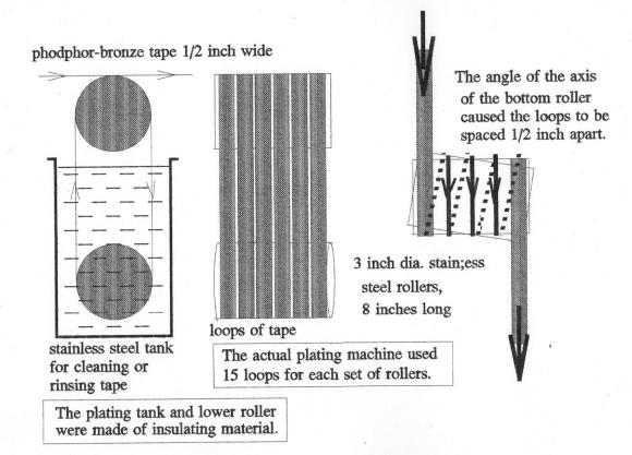
The tape was moved at a speed of around six inches per second [twelve for the second machine] by a motor that turned the top roller [or rollers] over the electroplating bath. The take up spool was turned by a motor with enough torque to just keep the spool turning. Also several roller stations before the plating bath were powered by motors controlled by sensors in order to prevent damage from excessive tension on the tape.
