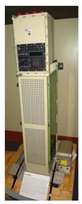
At the left is the CP-2044 computer donated from the Clearwater, FL factory. This unit represents our extended history of airborne computer systems since 1963. This unit was designed in the early 90's with embedded microprocessors to replace the CP-901 computers aboard the Lockheed P-3C. The Club's portable display below provided details of that history<sup>5</sup>, shown previously at the Club's annual picnic. [The 'Hunt for Red October' movie made the P-3C plane's prowess public.]
