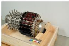
Runtime memory, mercury delay line UNIVAC I
