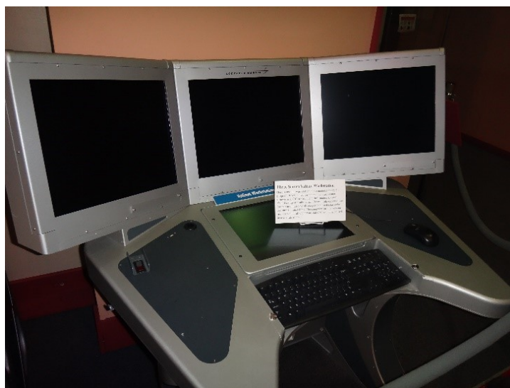
Picture 10. Designed in Eagan in the mid-90's, the AN/UQ-70 is the Navy's 5th generation computer system. These multi-screen demonstration units were donated by LMCO. Thanks to Legacy Committee Co-chair John Westergren.
