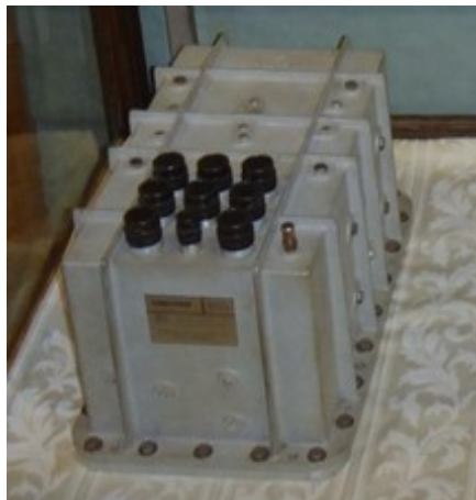
Picture 18. A missile 'onboard' guidance computer, UNIVAC type 1824 designed and built for the AF in the late 60s.
