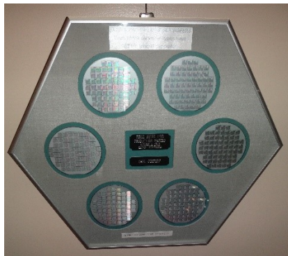
Picture 9. Each silicon wafer had 63 die, 1.25-micron lithography.
