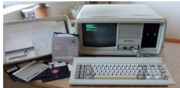
Picture 21. Two suitcase portable computers, circa 1975. These booted and operated from floppy discs.
