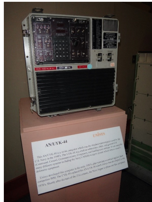
Picture 16. AN/UYK-44, the Navy's 4 th generation small scale shipboard digital computer, designed in Minnesota then manufactured at the Clearwater, FL facility.
