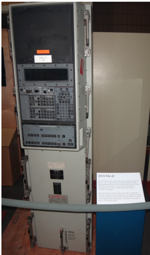
Picture 12. AN/UYK-43, US Navy's fourth generation standard computer for combat information centers, floor space is the same as the predecessor AN/UYK-7. On indefinite loan from U.S. Navy.
