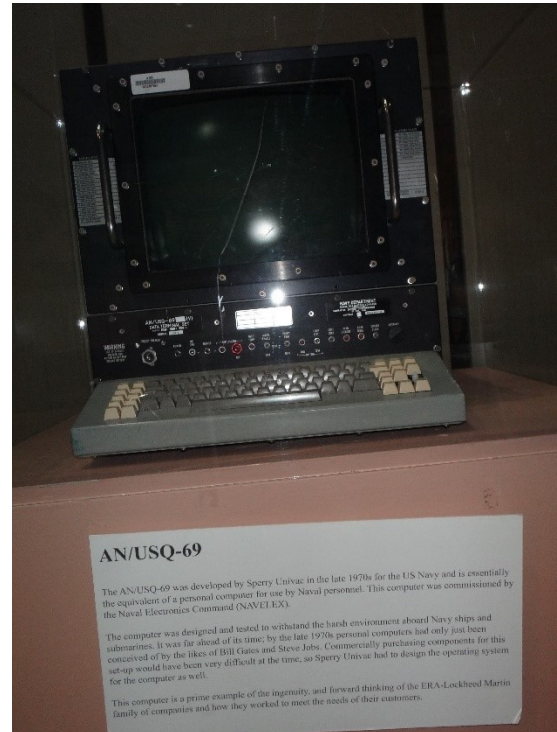
Picture 15. AN/USQ-69, the Navy's shipboard 'Personal Computer' developed by Sperry for NAVELEX in the 70's, also on indefinite loan from the U.S. Navy.
