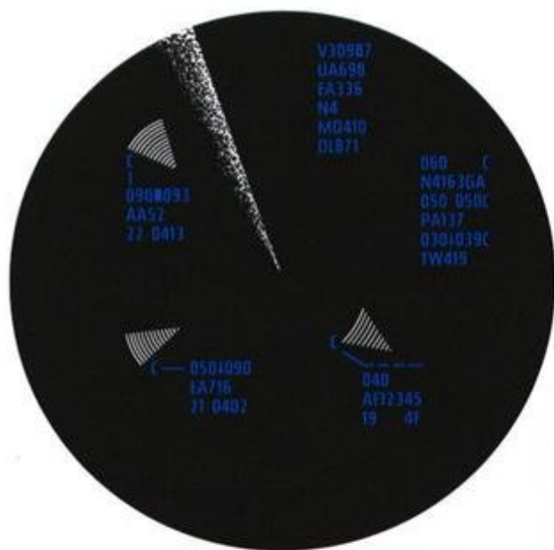
Fig. 1 — Computer-controlled alphanumeric flight data is superimposed over normal video on the controller's radar scope. The three alphanumeric "tags" shown in this illustration are automatically following radar and beacon video returns. Relocatable data tables (upper right quadrant) display pending flights and aircraft in holding patterns. (Video map, ground clutter, interference, and noise, which complicate the real radar display, have been omitted for clarity.) Fig. 2 (below) shows the two information paths to the display equipment: a direct video path that provides sensor data in the normal manner; and a digital path, via the computer for alphanumeric data.
