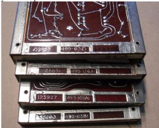
These are 4.5" x 6", with  $\sim$ 33 pin connectors. The P/Numbers at the left are most likely Assembly Part Numbers, stamped at the right are manufactured dates, i.e. 58 0401. What is the center 495-... number?
