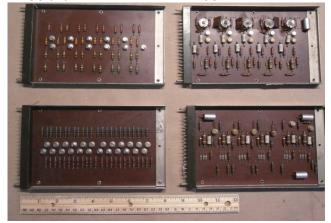
From the transistor count, the bottom left board looks like 12 Resistor-Transistor Logic flip-flops. The top right looks like pulse transformer circuits, either
