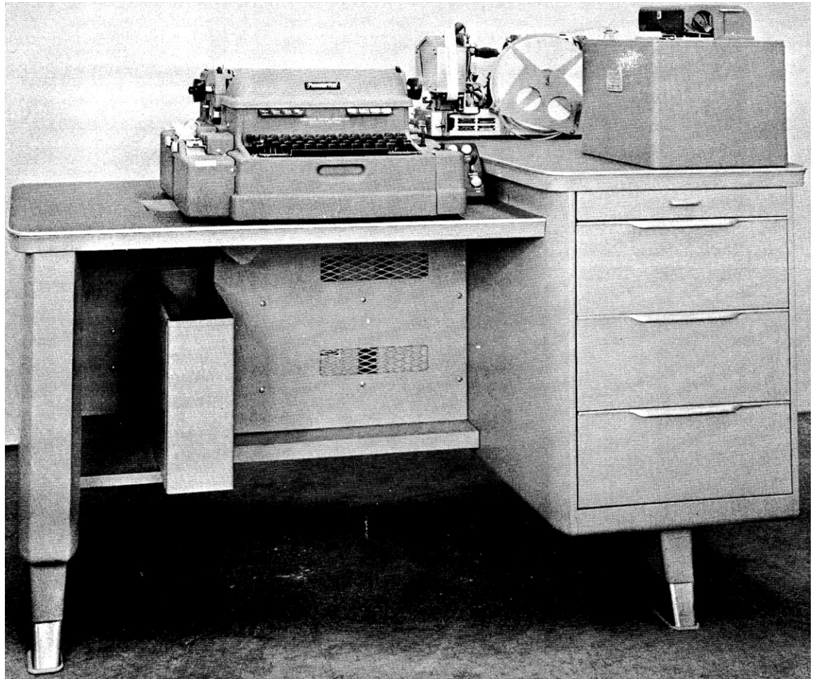
BuShips Computer - Input-Output Cabinet
