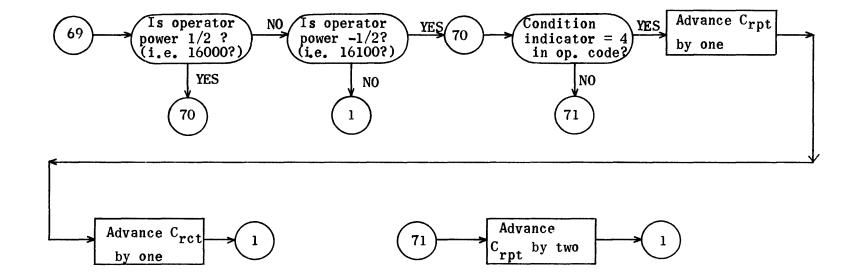
Equation Redundancy Check (Floating Point Divide and Subtract Operators)
