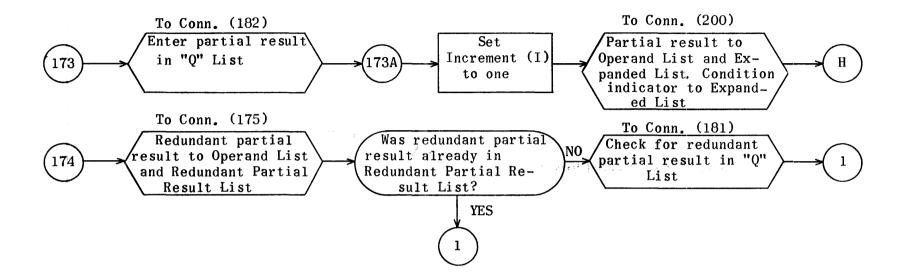
(RS) Subroutine to Store Redundant Partial Result in Operand List and Redundant Partial Result List.
