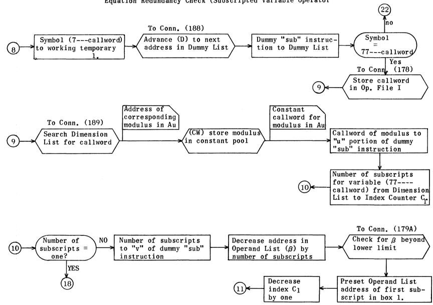
Equation Redundancy Check (Subscripted Variable Operator
