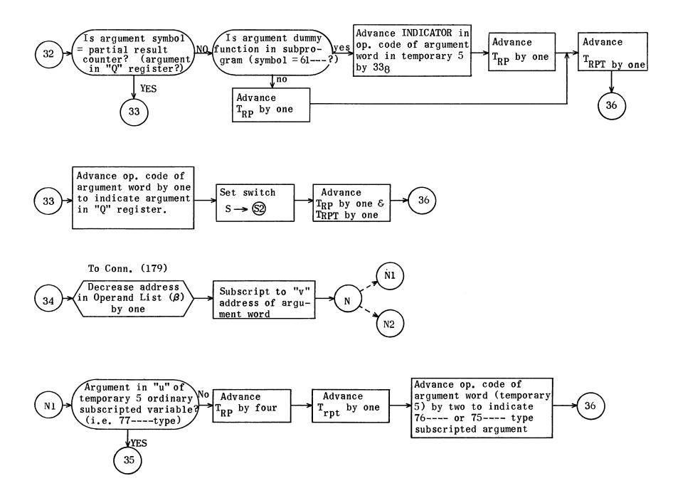
Equation Redundancy Check (Library Routine Operator)
