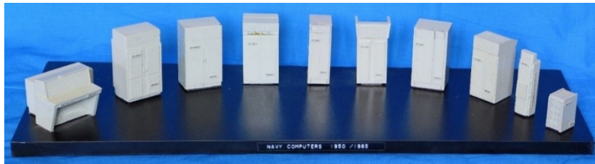
Figure 2. Models of NTDS 1 st and 2 nd generation computers at the Lawshe Memorial Museum – scale 1" = 1 ft. AN/USQ-17, CP-642A, CP-642B, CP-667, CP-789, CP-808, CP-848, CP-890, and AN/UYK-7. Germanium transistor machines were the Q-17, CP-642A, and CP-789. Silicon transistor machines were the CP-642B, CP-808, and CP-848. 2 nd generation CP-890 and UYK-7 used integrated circuit technology. The 1962 CP-667 used a combination of silicon transistors and integrated circuits.
