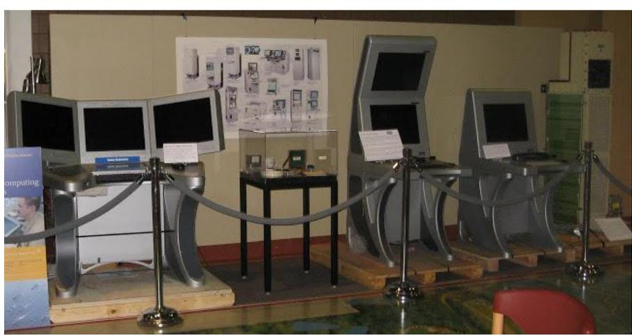
This photo at the left shows three variations of the AN/UYQ-70 workstation with embedded micro-processor units. The Q-70 is the 4<sup>th</sup> generation Naval Tactical Data Systems<sup>4</sup> (NTDS) standard computer.
