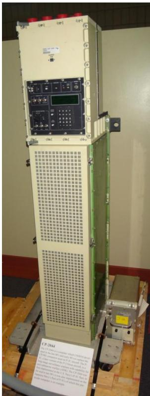
At the left is the CP-2044 computer donated from the Clearwater, FL factory. This unit represents our extended history of airborne computer systems since 1963. This unit was designed in the early 90's with embedded microprocessors to replace the CP-901 computers aboard the Lockheed P-3C. The Club's portable display below provided details of that history<sup>5</sup>, shown previously at the Club's annual picnic. [The 'Hunt for Red October' movie made the P-3C plane's prowess public.]
